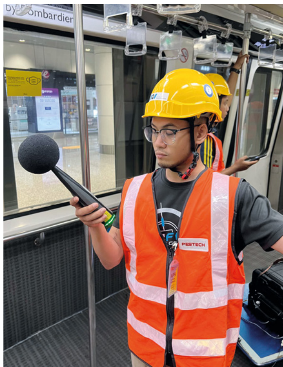
Noise testing inside aerotrain.
